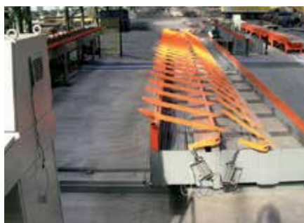
6. CPO: Mobile optimizing roller carriage. For storing and transferring bundles of bars cut to size towards subsequent machining operations.
