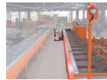
9. CC: mobile commissioning carriage. To unload the cut bars onto the floor classifying them in specific deposits.
