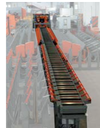
14. VS: unloading track. It has the function to receive the bars from measuring and transfer track (VMT) aligning it and to unload the bars on the storage sections.
