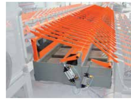
8. T: Storage optimisers. Allows completion and lengthwise transfer of bundles of bars requiring subsequent bending.
