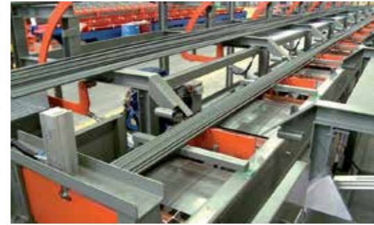
2. VA: Pre-storage system with rotating arms on entry conveyor
