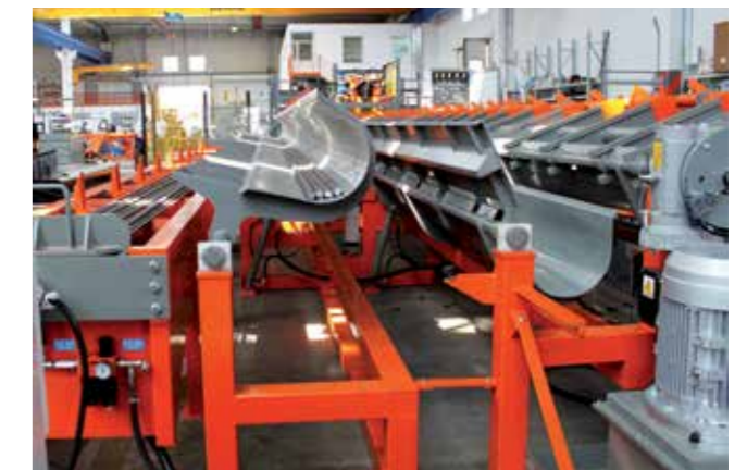
16. Lifting buffer. It receives the bars from the Shearline pockets and lifts them onto the roller track of the bending robot.
