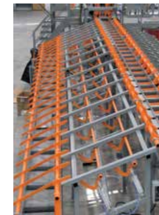
15. SDS: Pneumatic storage slide. Slide with 2 pneumatic arms for bars collection, able to transfer the bars to the close bending bench or bending robot.
