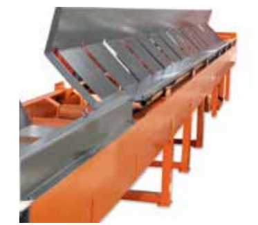
10. VRP: distribution tracks. They allow storing cut bars and act as storage unit for subsequent working operations.
